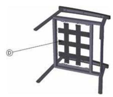
**D:** Place the chair frame on the floor. Take a pair of scissor and cut the seat webbing straps at the point where the hook connects to the webbing. Separate the webbing and hooks.
