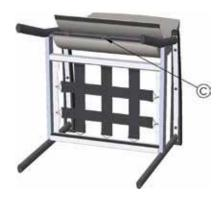
C: Using a #2 Philips screwdriver remove the back(s) (six screws each).
