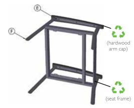
**E&F:** Using a #2 Philips screwdriver remove each arm cap (three screws). Using the pliers, remove each the glide from the bottom of each leg.
